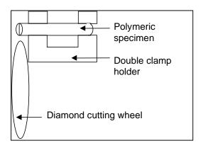
Figure 1: Illustration of the cutting arrangement used for sectioning the polymeric material. The sample was clamped onto the machine using a Model 65003 Double Clamping Holder and sectioned using a diamond wheel.
